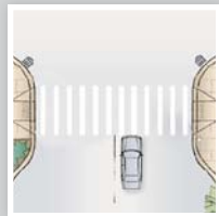
02 High visibility crosswalks (5.1)
