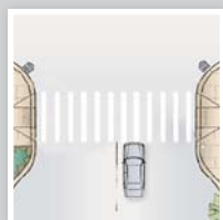
02 High visibility crosswalks (5.1)
