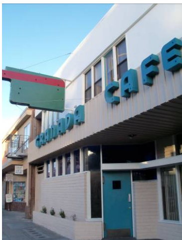
Left: Painted sheet metal individual letters of the Granada Cafe, built in 1949, on Mission Street in the Excelsior District. This largely intact storefront features additional Midcentury Modern design elements including a recessed, asymmetrical entryway, overhangs, brick veneer, and planters integrated in the building's façade. Right: The Butler Brothers department store (1952) at Stonestown featured a "billboard facade" with script lettering readable from an automobile. Photos: Mary Brown, San Francisco Planning Department; San Francisco History Center, San Francisco Public Library
