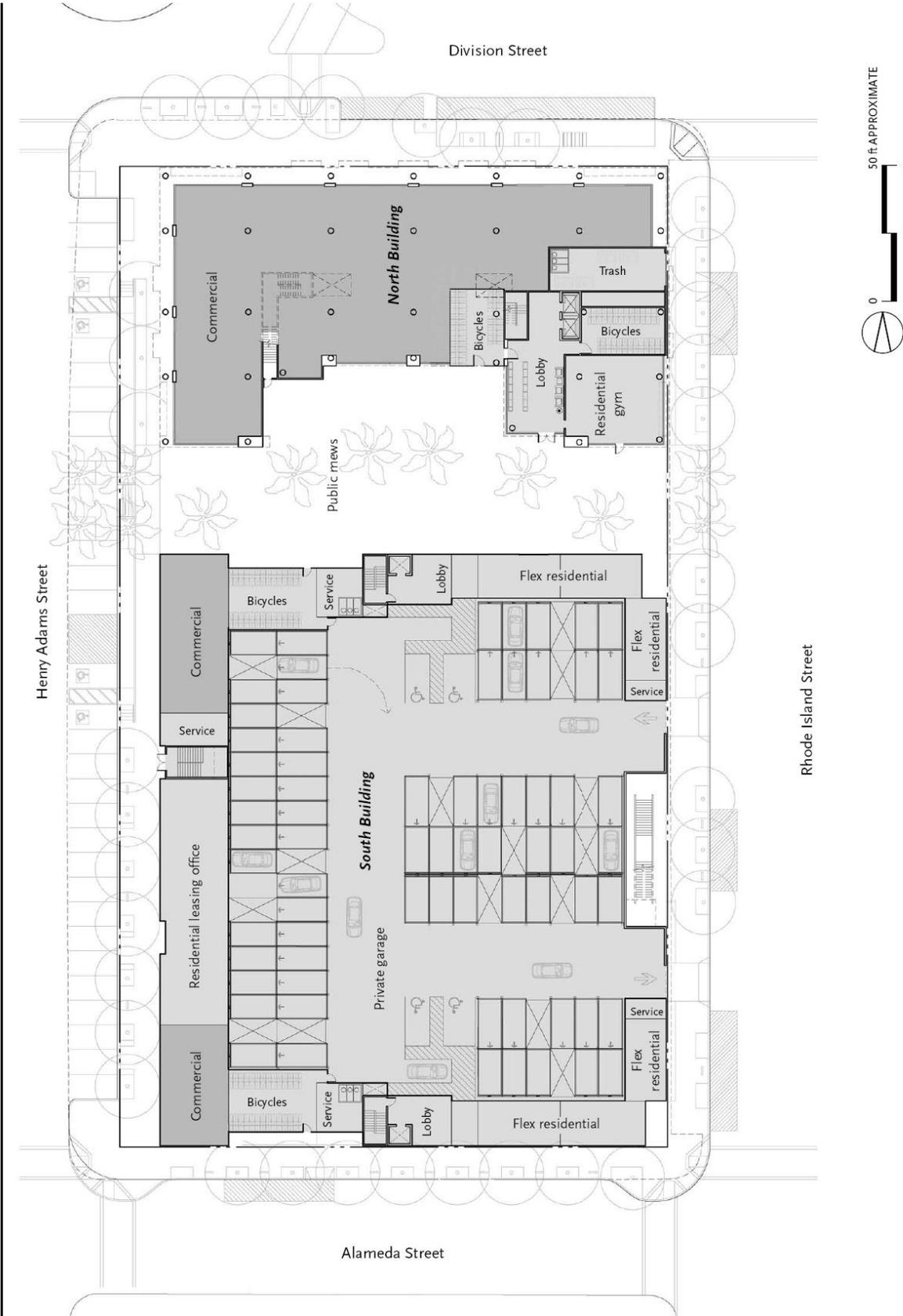
Variant 3: One Henry Adams Site — First Floor Plan Figure RTC 7
