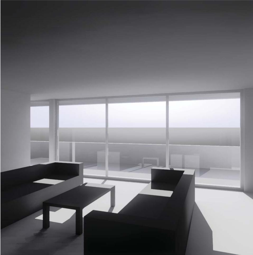
Even with a 6' overhang that increases thermal performance, additional movable shades, either inside or outside the glass, will be useful to manage the brightness of the sky and deep sun penetration in the afternoons. This is an image created in *RADIANCE* that simulates the view looking to the west from the penthouse at 4:00pm on March 21.
