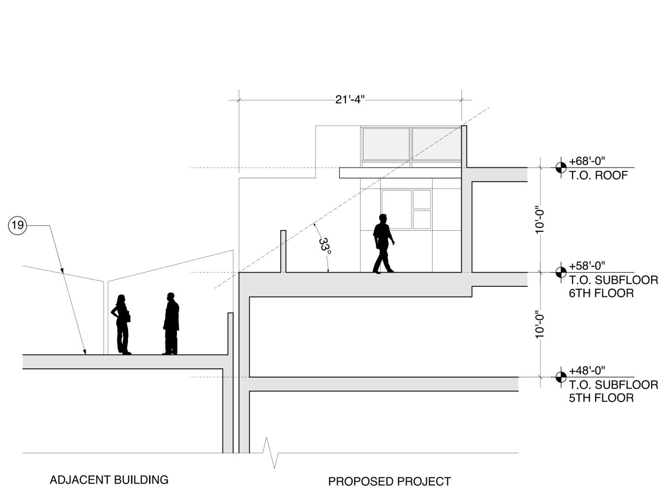
SECTION THROUGH ROOF DECKS LOOKING EAST 2
