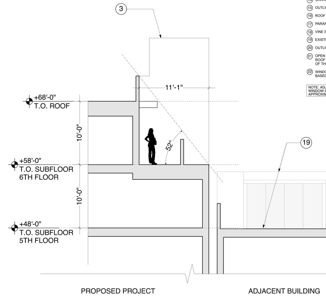
SECTION THROUGH ROOF DECKS LOOKING WEST 1
