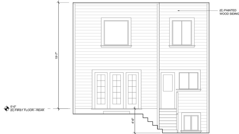
3 EXISTING SOUTH ELEVATION - REAR FACADE
