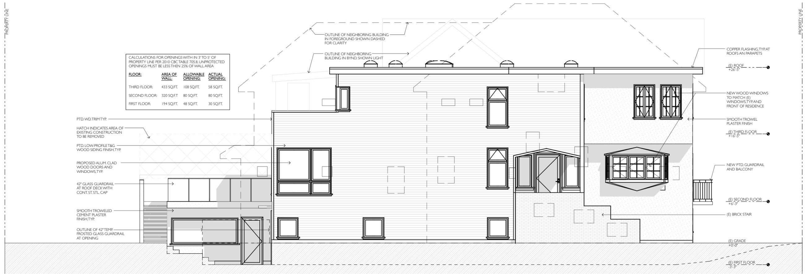
CALCULATIONS FOR OPENINGS WITH IN 3" TO 5" OF PROPERTY LINE PER 2010 CBC TABLE 705.8, UNPROTECTED OPENINGS MUST BE LESS THAN 25% OF WALL AREA
