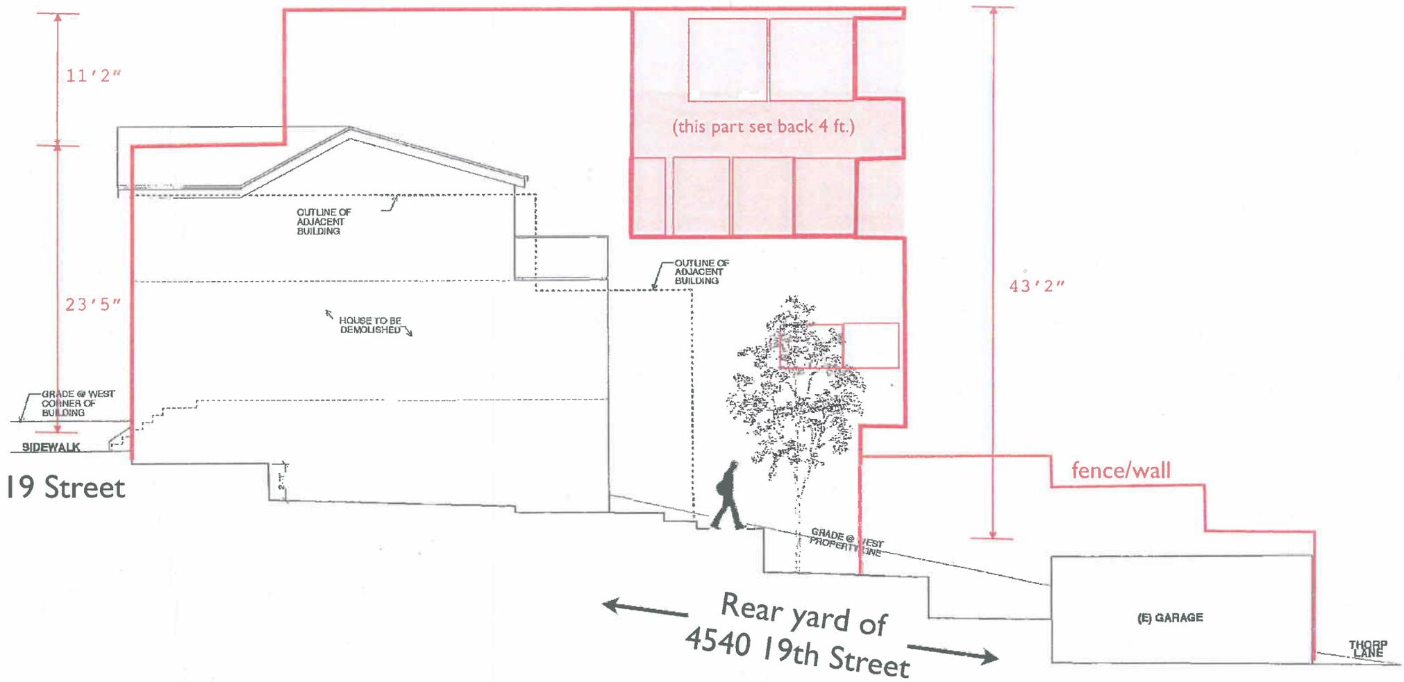
Side view, facing adjacent downhill lot at 4540 19th Street, of the proposed structure (drawn in red) superimposed upon the existing structure (black). All objects are drawn exactly to scale from plans provided. Walking man is 5'10".
