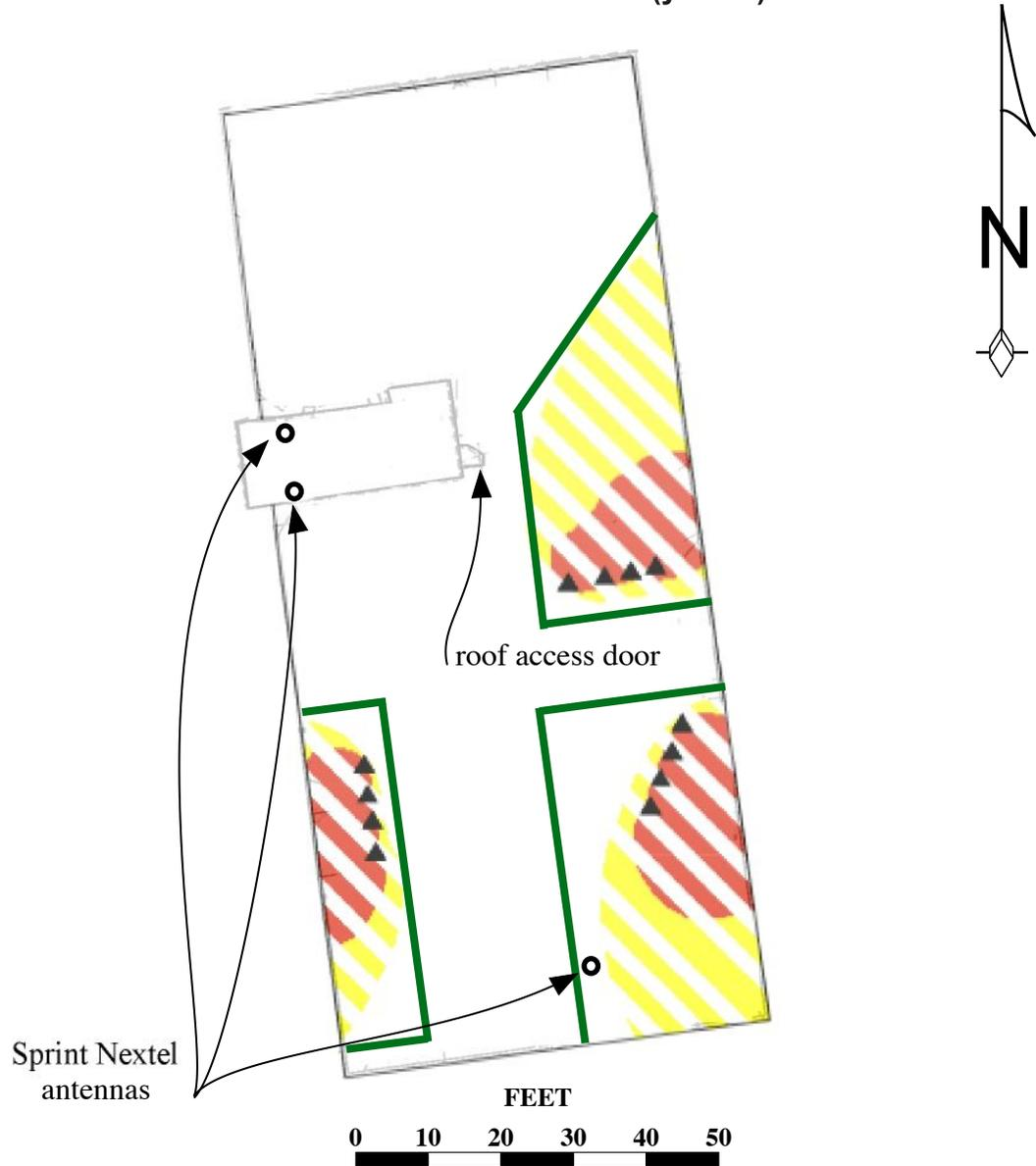
Calculated exposure levels and barricade locations shown are based on contribution of AT&T only.
