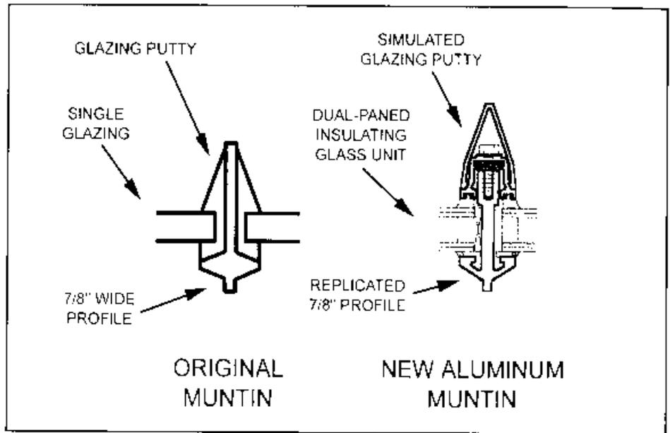
Figure 5. The replacement aluminum muntin accurately replicated original profiles while accommodating insulating glass and thermal stops. Drawing: Bruner/Cott and Custom Window.
