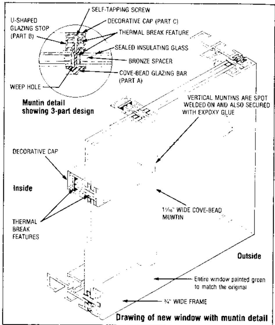
Figure 3. Drawing of the aluminum replacement window shows how the cove-bead muntin profile of the original steel windows was closely matched in the integral muntin system designed for the aluminum replacement window. A series of spacers and gaskets were used as the principal means of obtaining a thermal break in the window for energy purposes. Drawing: Peter Charles
