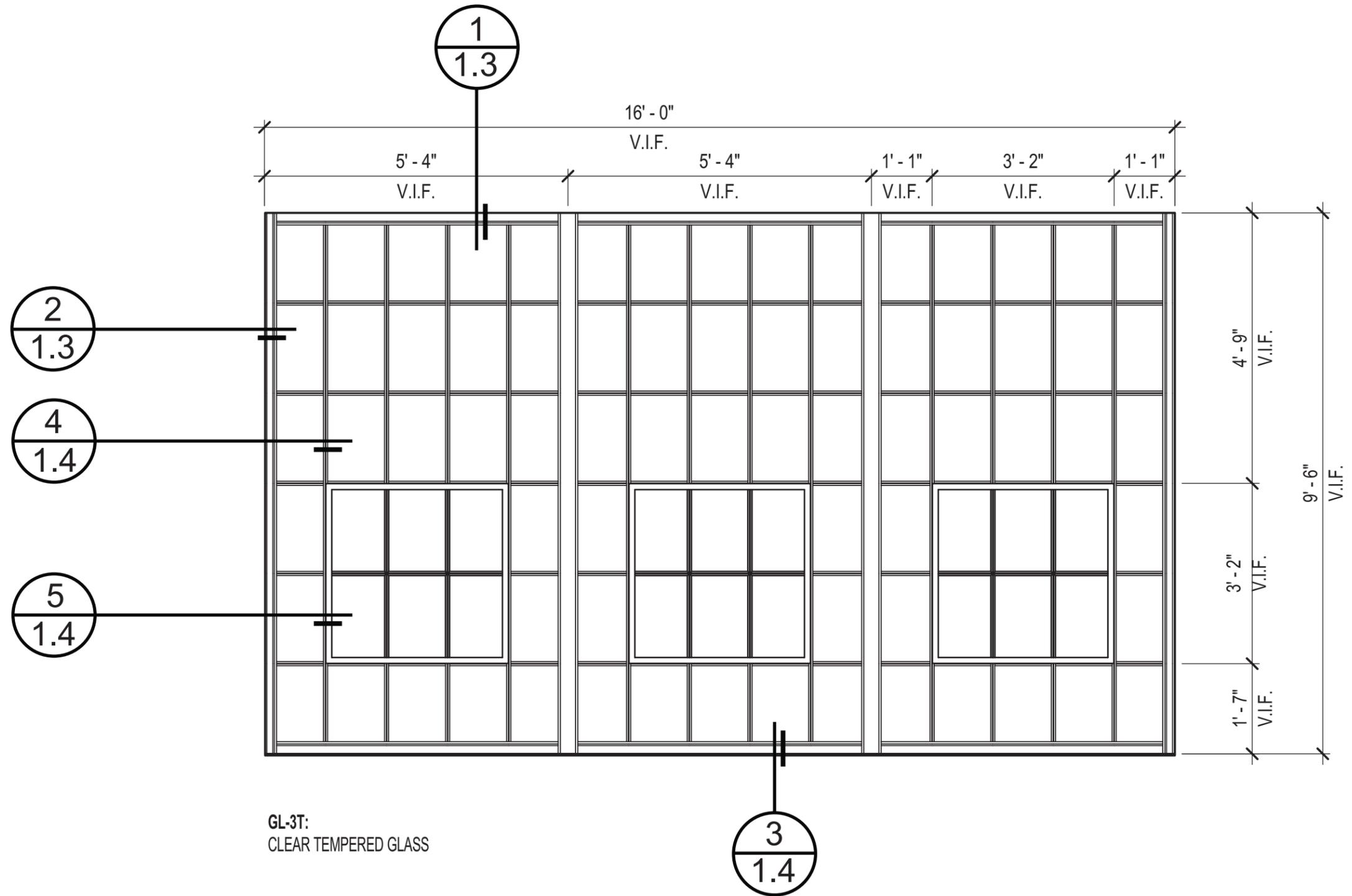
**ALUMINUM REPLACEMENT WINDOW - TYPICAL - ELEVATION**
