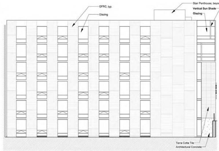
Figure 13: North Setback Elevation
