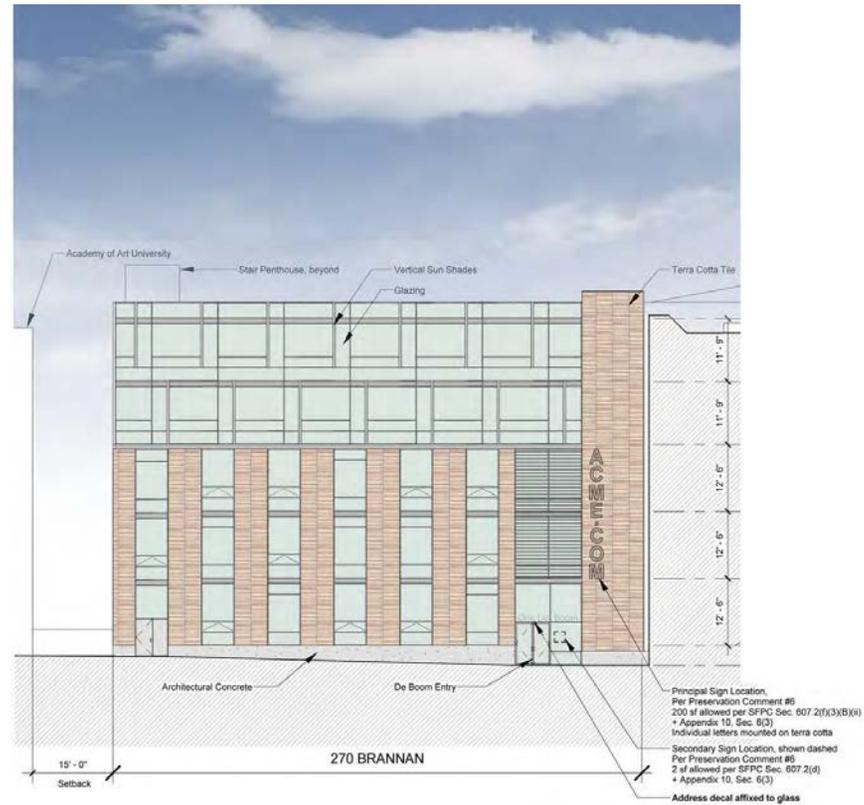
Figure 12: De Boom Street Elevation
