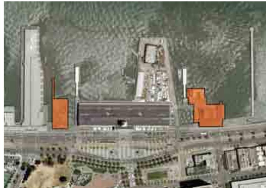
**Deck and Piles in Poor Condition.** In the North Basin, Pier ½ was red-tagged in 2010. In the South Basin, Pier 2 and Sinbad's as well as the substructure of the Agriculture Building was identified as being in poor condition.
