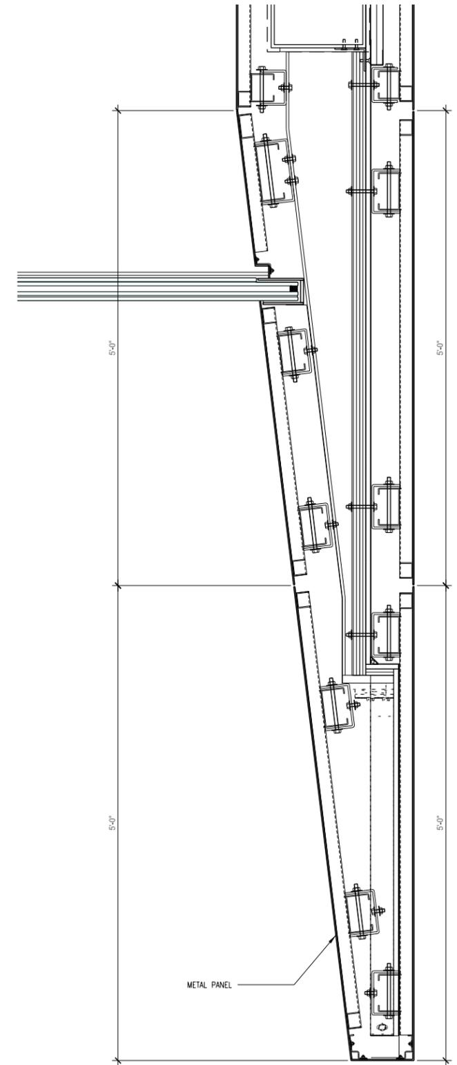
02 EXTERIOR STOREFRONT CHAMFERED FRAME PLAN DETAIL
