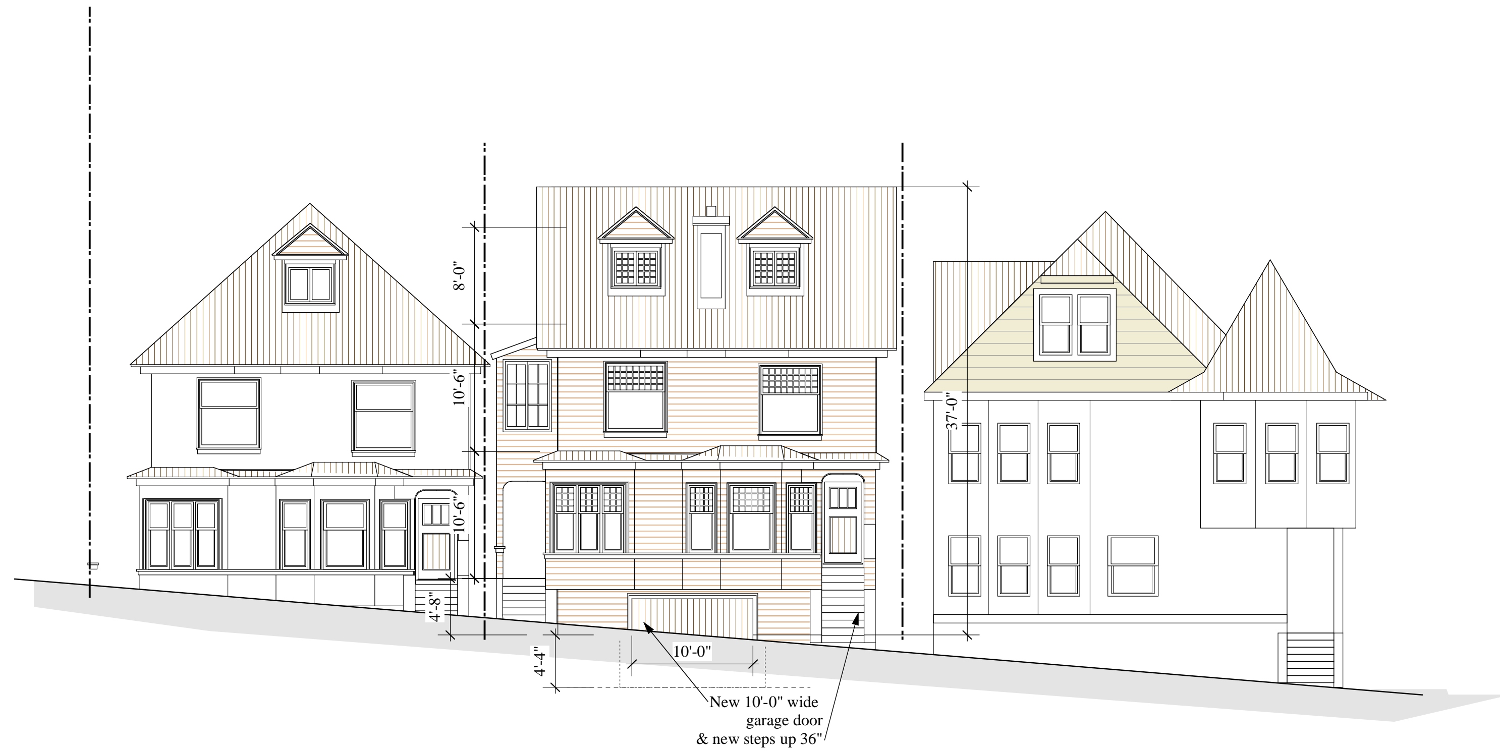
B A5 NEW ELEVATION- 2853 & 2857 BRODERICK (raised 36") Scale: 1/8" = 1'-0"
