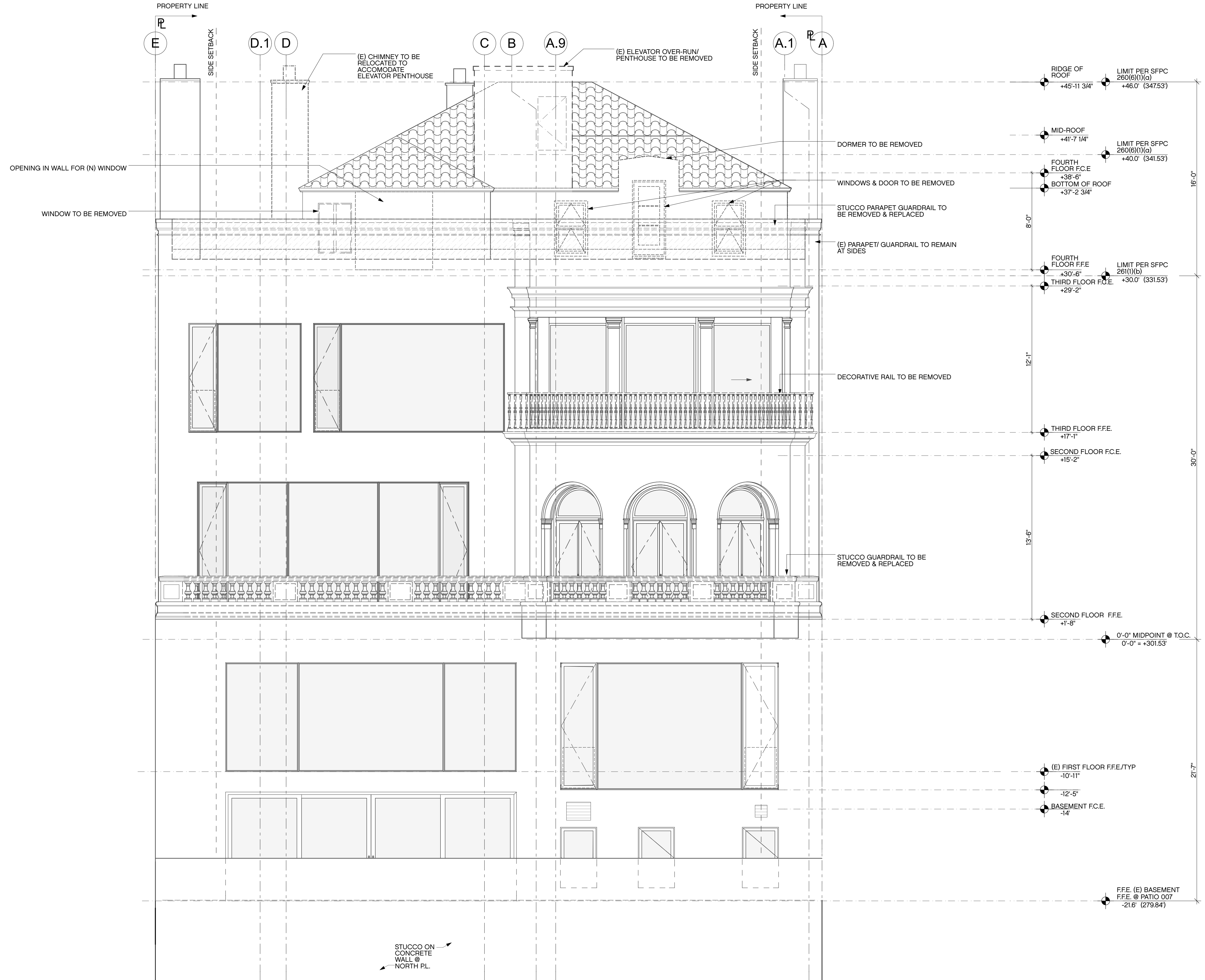
1 NORTH DEMO ELEVATION SCALE: 1/4" = 1'-0"
