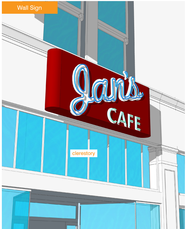
New wall signs must be mounted on a flat surface of the building and must not block more than 50% of any clerestory/transome window.
