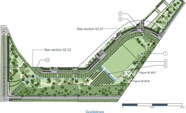
02.20.05 Pedestrian Path A continuous 6 foot pedestrian path must follow the flow line of the stream corridor, connecting Juan Bautista Circle to Belvedere garden. A clear system of wayfinding devices must be incorporated into the design of the path, especially at intersections with streets.
